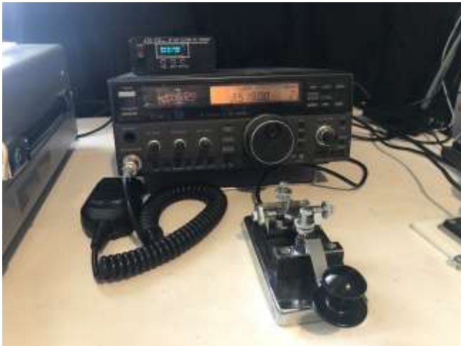
Rig set up for CW on 80m band – 3519kHz
